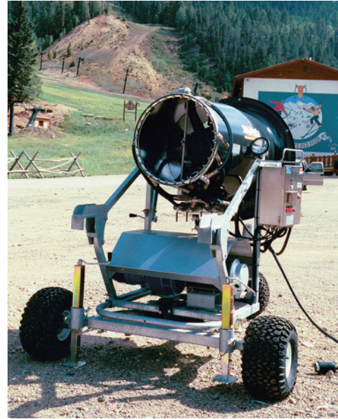
Figure 1-7 Snowblowers can produce artificial snow by evaporative cooling. (Courtesy of Red River Ski Area)
